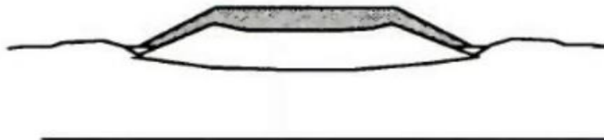
Figure 1.9. Punching under an embankment (Dadouche [23])
