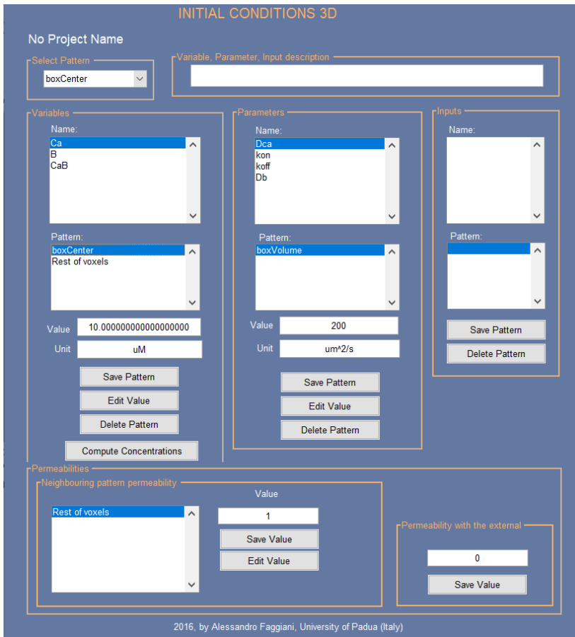
Figure 2.4 Initial Condition panel: starting value of 'Ca' variable is defined in the pattern "boxCenter" and in the "Rest of voxels". Value for Dca coefficient is defined in the whole box volume.
