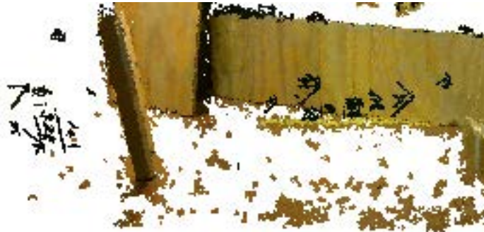
Figure 4.26: Detail of dense reconstruction for the office sequence. Some patches of noise are visible
