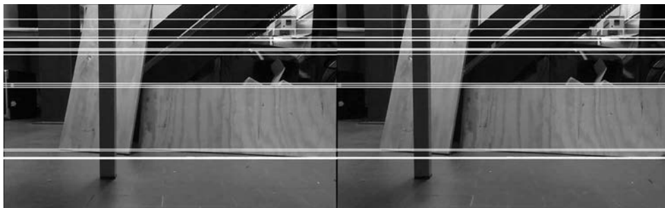
Figure 4.16: Images of the office sequence with epipolar lines, rectified and correctly centered.
