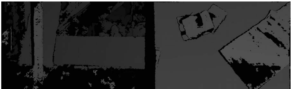
Figure 4.21: Frames densely matched with a block size of 7
