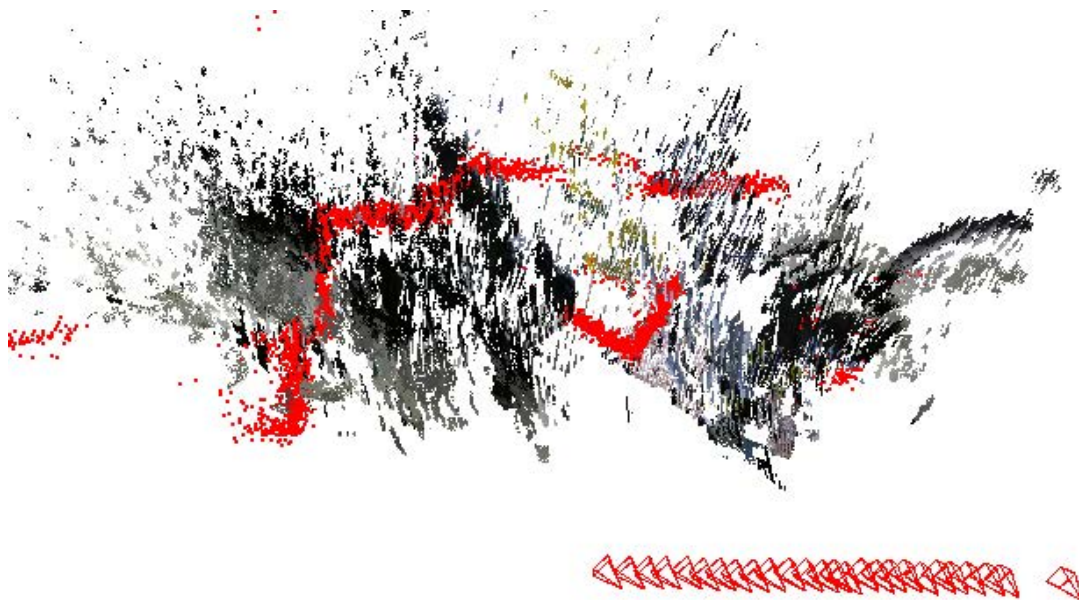
Figure 4.103: Corridor 45° dense clouds and LiDAR cloud seen from above. View 3.
