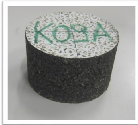
Figura 25: provino Marshall additivato
