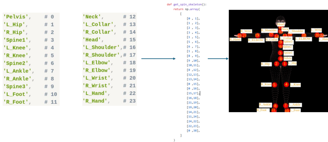
Figure 2.3: The left image represent SMPL joint ids to joint names, the middle one represent unique joints connectivity each method use (SPIN for us) and with that we can visualize a Kinematic tree shown in the right image
