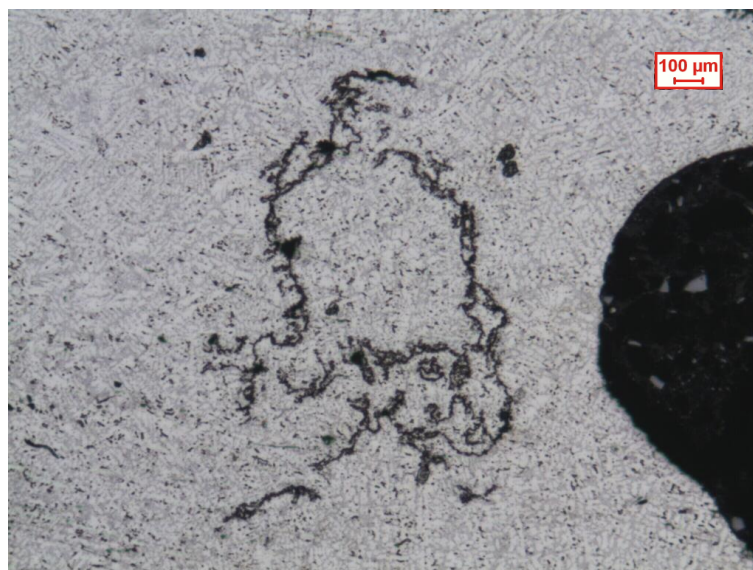
Figure 1.8: Tangled oxide film.
