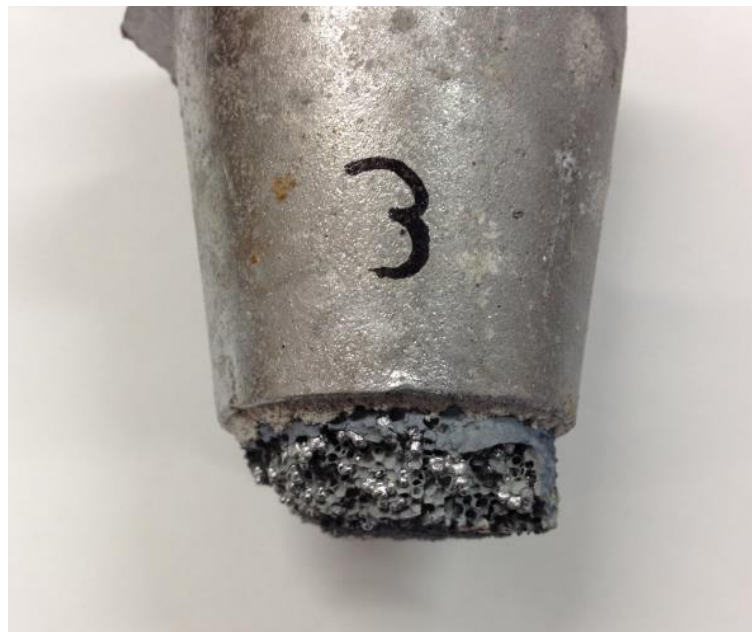
Figure 2.3: Filter filling failure.
