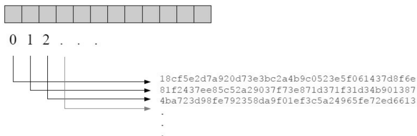
Figure 2.2: Example of hash computation for every piece composing a torrent.
