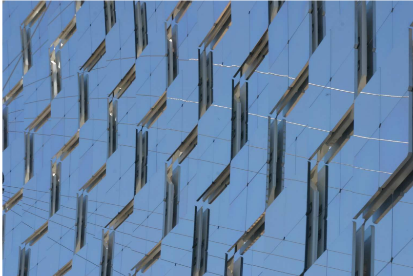
Figure 2.5: Photo of the reflectors of MAGIC I, from [9]. It can be noticed that the mirrors are grouped in panel composed by 4 elements.
