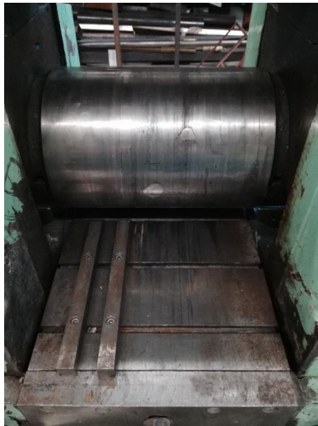
Figure 2.2: cold rolling machine used in BME, Budapest (a) and a schematic representation of cold rolling process (b)
