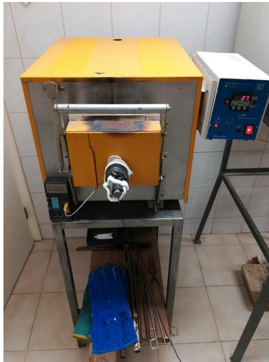
Figure 2.15: set-up of AE furnace
