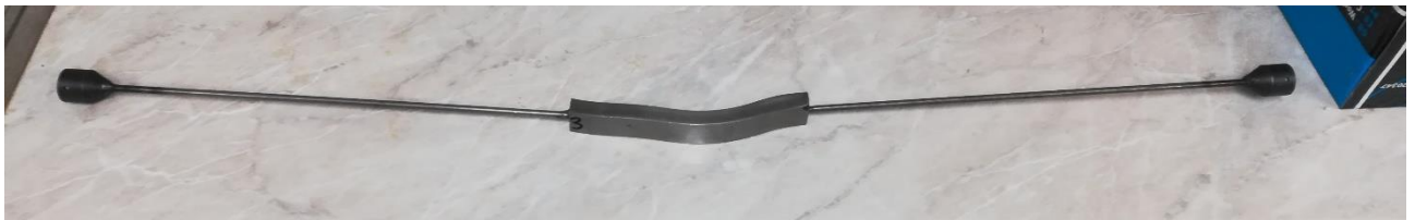
Figure 2.13: First configuration - two small rods connected to 304 rolled sample
