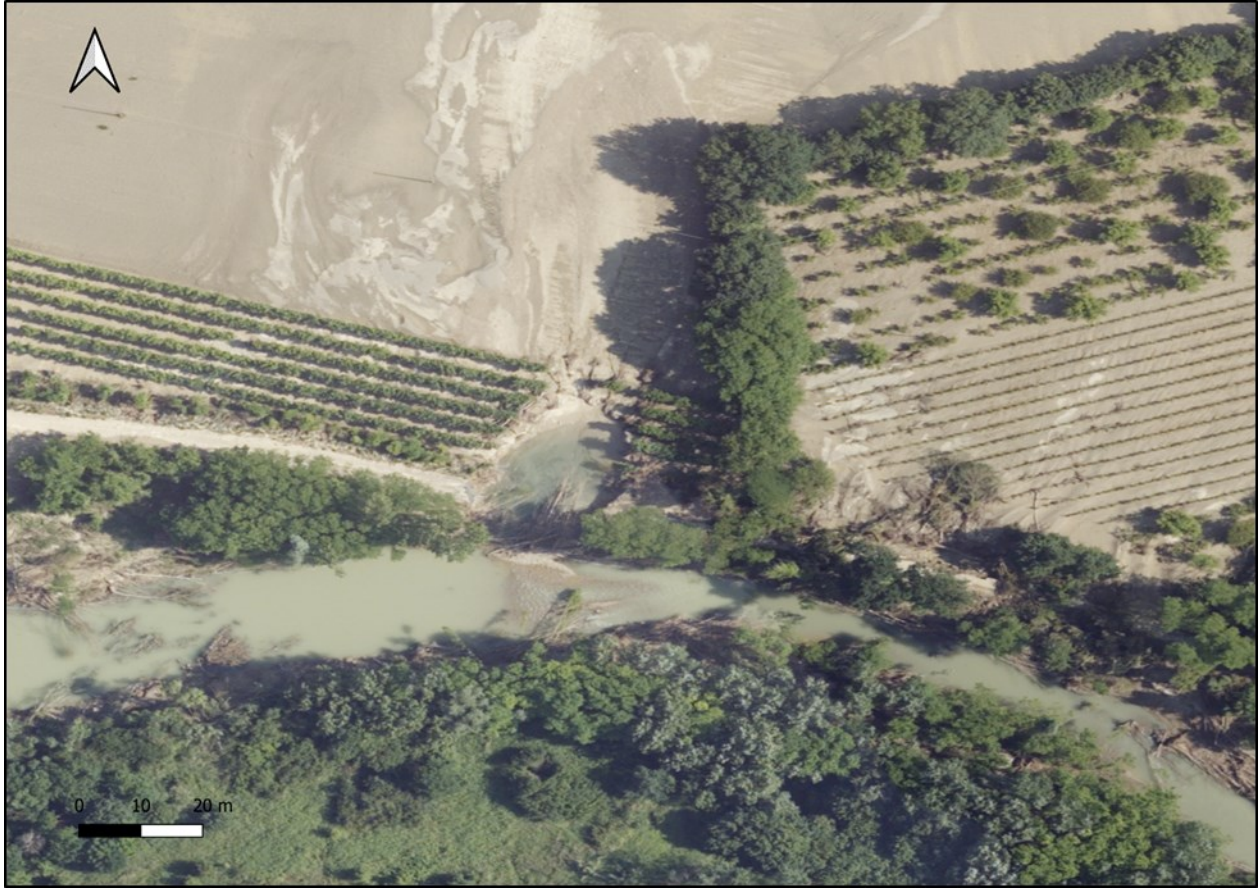
Figure 6.3: Observed overflowing location at meander part of Senio River
