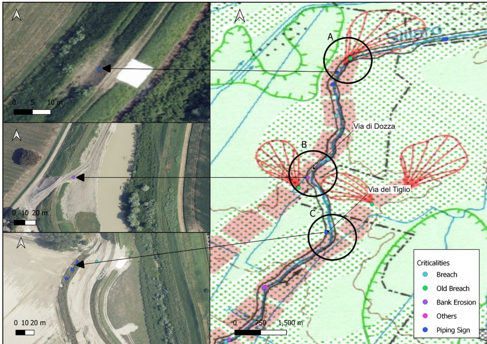
Figure 6.13: Geomorphological Map overlaid with criticalities observed from post May 2023 event orthophoto (Sillaro River)
