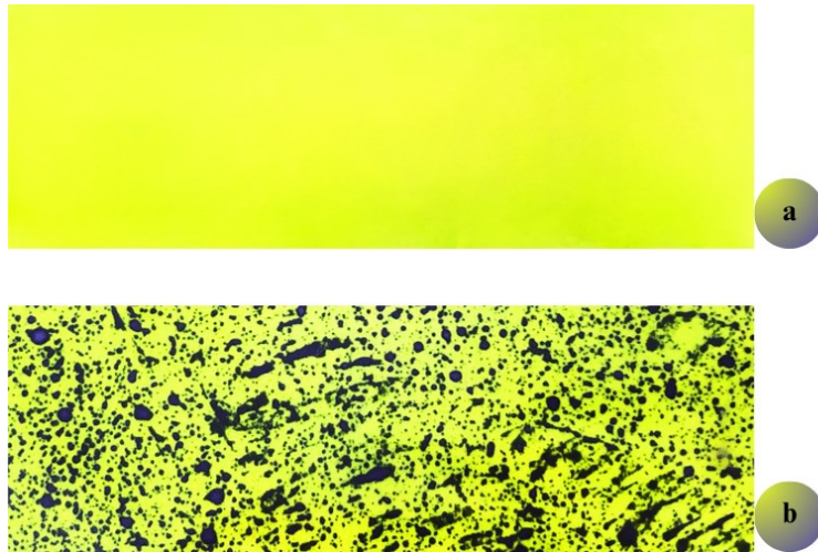
Figure 4. WSP before exposure (a) and after exposure (b) to the spray.
