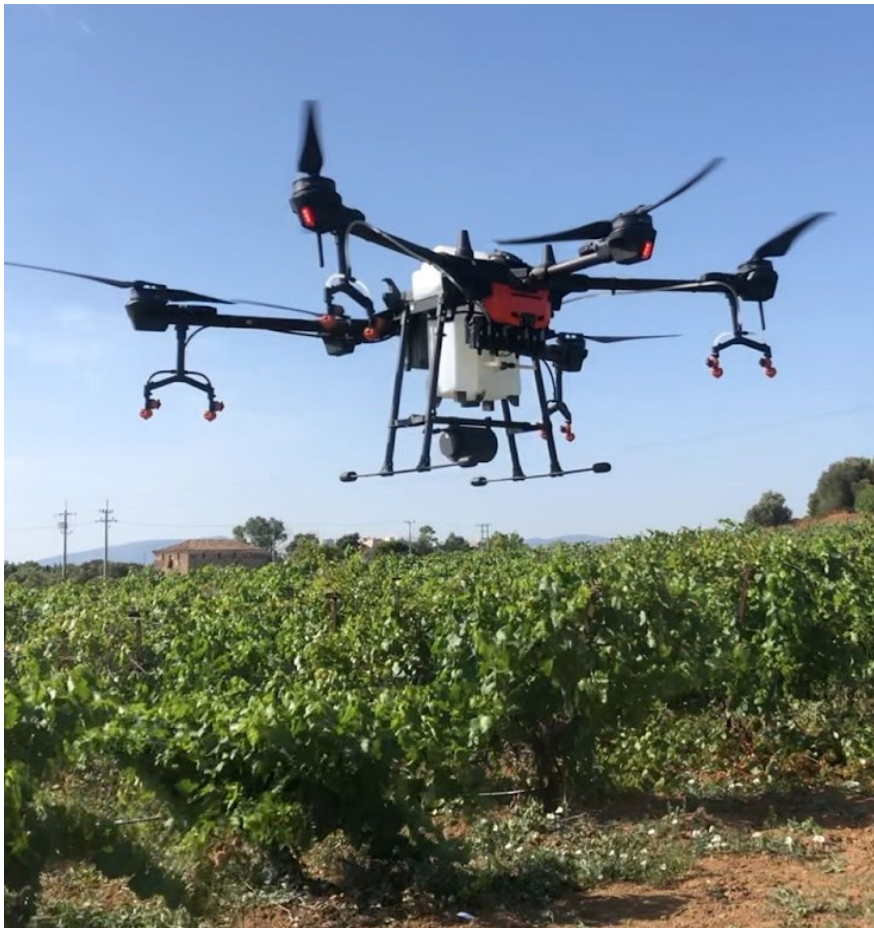
Figure 2. The multi-rotor (hexacopter) UAV used in the spraying experiment, DJI Agras T16.
