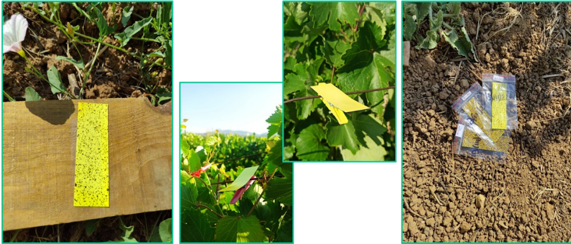
Figure 6. Photos from the experiment showing Ground WSP, Canopy WSPs and zip lock bags used.
