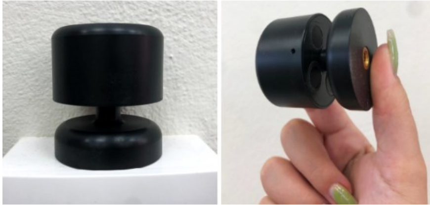
Figure 3. Ultrasonic Portable Mini Wind Instrument and Data Logger used in the spraying experiment.
