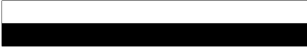
Figure 4.5 Representation of the geometry used in the numerical simulation using the software Comsol Multiphysics. The hydrofluoric acid a 40% weighted concentration is represented in white whereas the glass subdomain is depicted in black.
