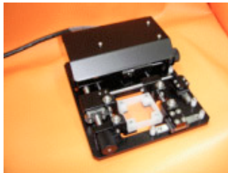
Figure 1.4 Stretch Apparatus (Strex) developed by B-Bridge International.
