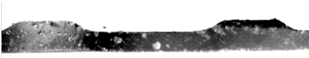
Figure 4.7 Cross section of an etched single channel acquired with a stereomicroscope. The channel width is 550\mu\text{m} and its depth, obtained after 3 minutes of reaction, is about 40\mu\text{m} .
