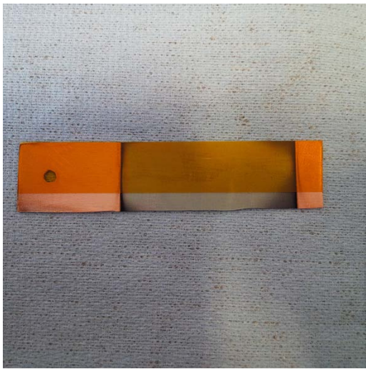
(a) First piece of insulating tape.
