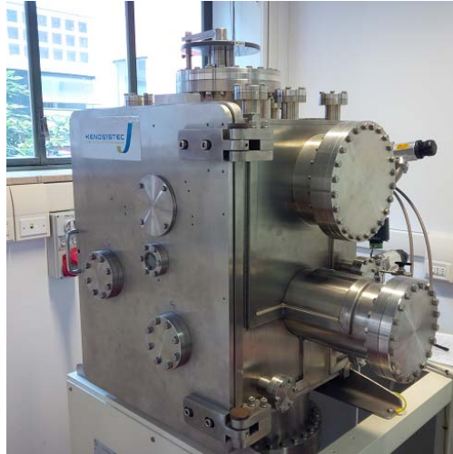
Figure 6.1: Magnetron sputtering system of the laboratory of Micro and Nanostructured Materials of the University of Padua
