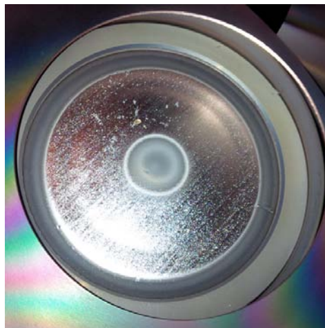
Figure 4.3: Aluminum (99.9999%) target used in the magnetron sputter of the laboratory of Micro and Nanostructured Materials
