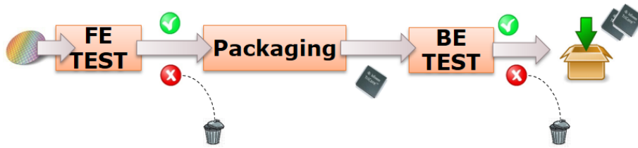
FIGURE 1.2: From wafer to chip: The process start with a wafer with hundreds of ICs, that goes through FE testing, the dies who pass the FE are packaged and sent to BE testing, the passing packaged chips are ready to be shipped
