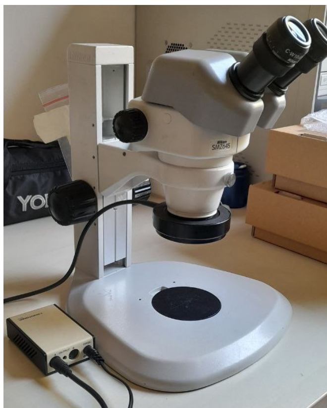
Figure 22 - Stereo Microscope Nikon SMZ645 with zoom range of 0.8x - 5x magnification present at Geoscience department of Padua University.
