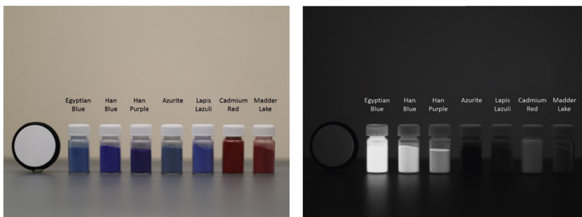
Figure 9 - Visible light image and VIL of some pigments (Modified after THAVAPALAN ET AL. 2016).
