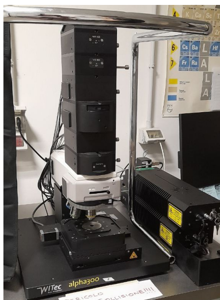
Figure 26 - Raman spectrometer WITec alpha300 R at the Geoscience department equipped with 532 nm and 785 nm lasers (left) and schematic diagram of Raman instrument (right) (CAMPANELLA et al. 2021).
