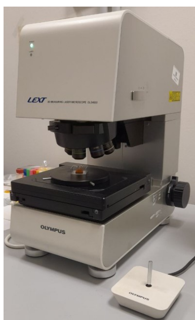
Figure 24 - Olympus LEXT OLS 4000 3D Laser Measuring Microscope in the Geoscience department of Padua University (left) and schematic representation of a confocal microscope. (ENCYCLOPÆDIA BRITANNICA, INC. 2024)
