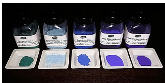
Figure 10 - Kremer Pigmente ©, in order from the left: EG, EB (particles < to 10 μm), EB (particles < 120 μm), CB and CP. Modified after (NICOLA ET AL. 2023)
