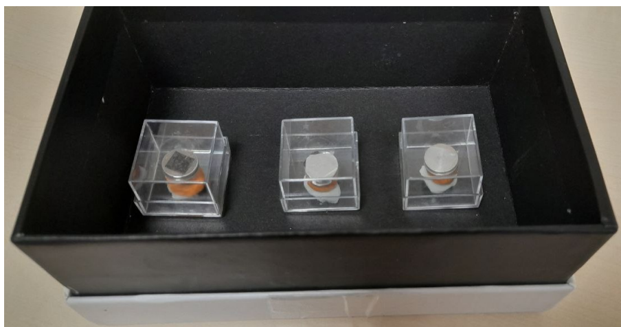
Figure 40 - From the left: sample No.1 on glass, sample No.2 on aluminium foil, sample No.3 directly on stub.
