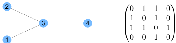
Figure 1.1: Given a simple graph G on 4 vertices, we see how it can be represented by a 4 \times 4 matrix.
