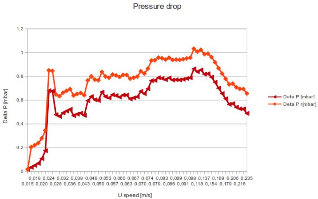
Fig. 2.25 Comparison between the pure signal (Delta P) and purified from noise one (Delta P r) (Glass spheres 12 \mu ).
