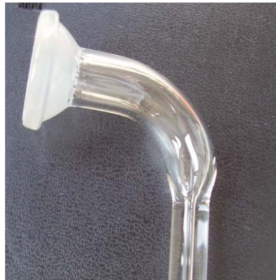
Fig. 2.20 Photograph of the top of the third prototype, the tube had to be enlarged in the ending part to permit the connection to the following separation system.
