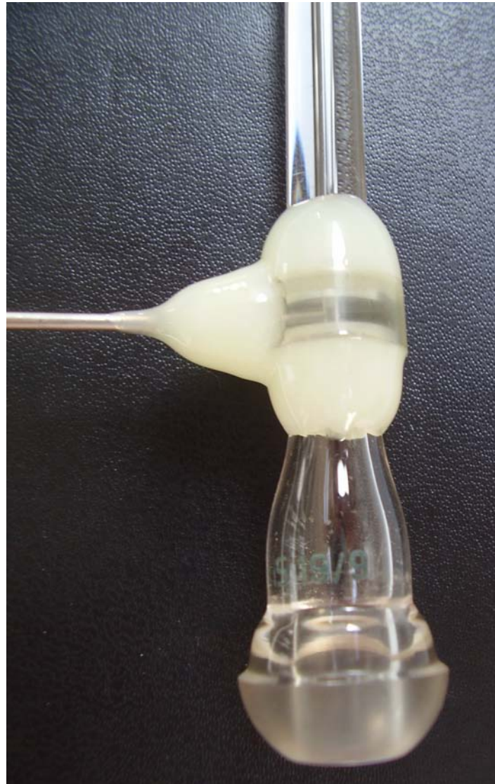
Fig. 2.21 Photograph of the bottom of the third prototype: installation of the connection piece with filter and pressure socket .
