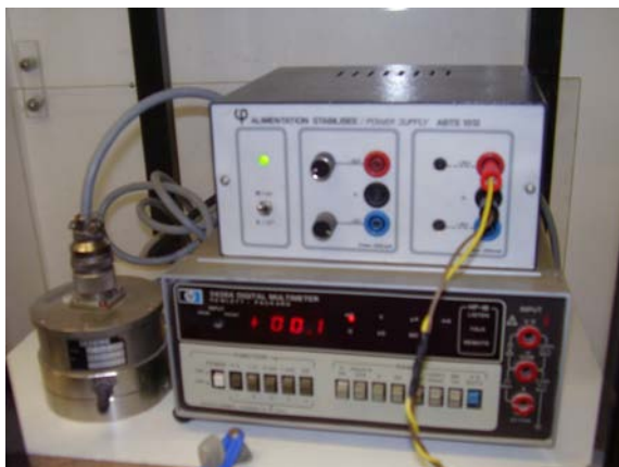
Fig. 2.22 Differential pressure sensor, its power supply and a connected voltmeter unit.
