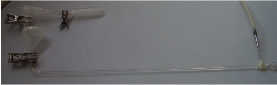
Fig. 2.18 Photograph of the third prototype; on the left side of the picture the separation system connected at the fluidization tube; on the right side of the picture the pressure socket connected to the measurement instrumentation.
