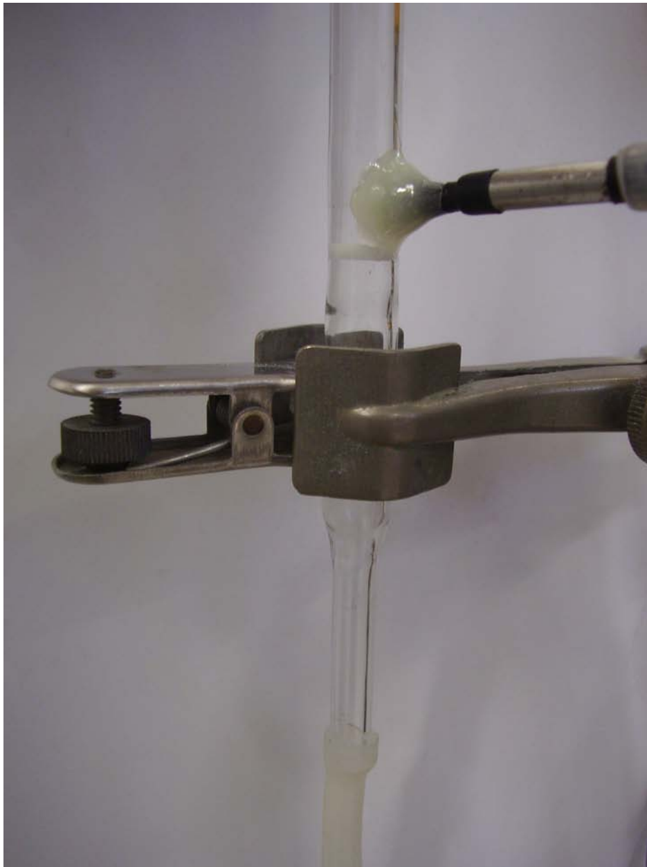
Fig. 2.11 Particular of the lower part of the apparatus: the compressed air inlet, the pressure socket and the porous glass filter.
