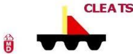
Fig. 6: Example of cleats designed to convey small products.
