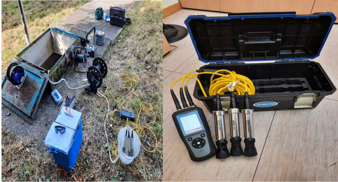
Figure 21. Setting and instrumentation used in water sampling procedure.
