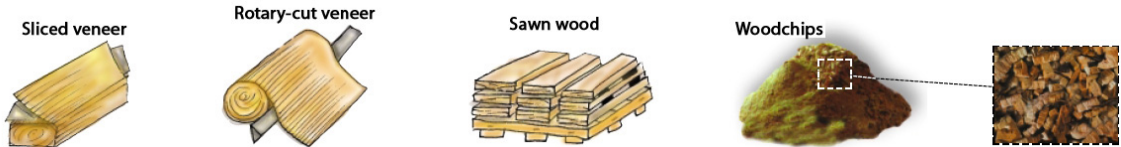
Figure 2.1: Timber assortments that can be obtained from tree-farming plantations (Buresti & Mori 2000, modif.).
