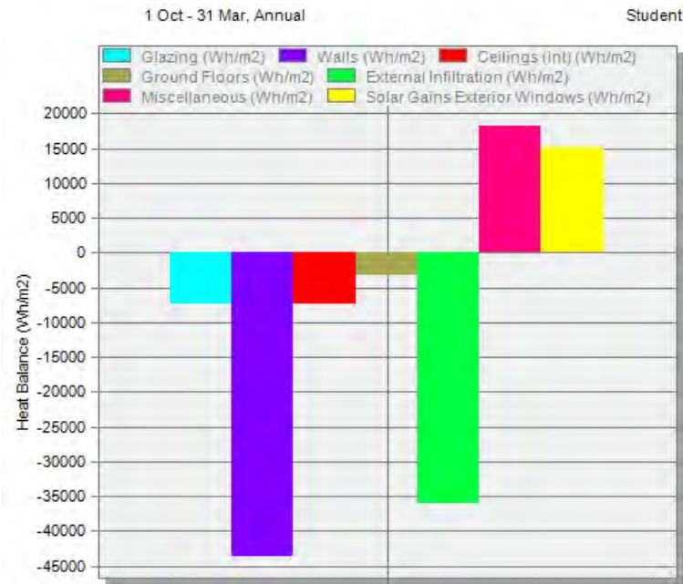
Figure 36 : Winter heat balance (source: Design Builder)
