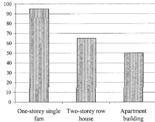
Figure 11: Variation in energy requirement for space heating ( \text{kWh/m}^2 ) between different housing types with 120 \text{ m}^2 of residential floor area. The figure applies to Oslo climate conditions (Duun et al. 1988)
