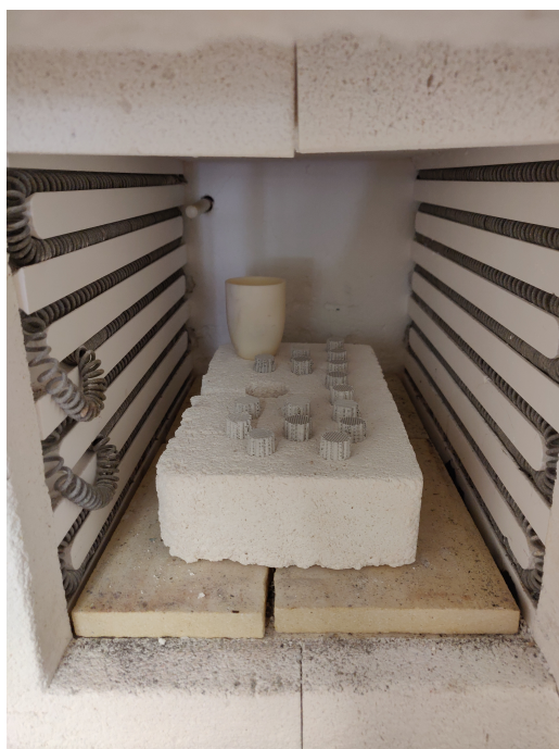
Figure 5.4: KGP-40HT and HT thermal treatment T6
