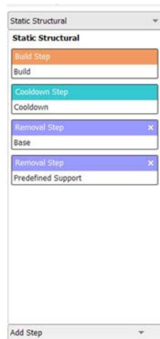
Figure 108- stages of the AM process simulation
