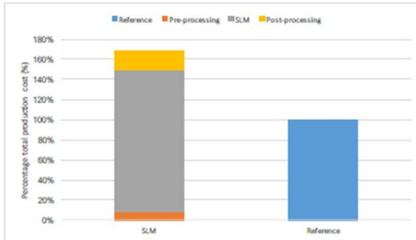
Figure 130- L-PBF production cost compared to conventional manufacturing cost
