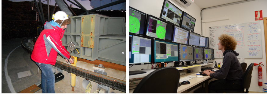
Figure 2.7: Two pictures of me working during the shift P136. Left: Removing a bolt which prevents the structure from moving due to strong winds. Right: Writing in the runbook the weather conditions.
