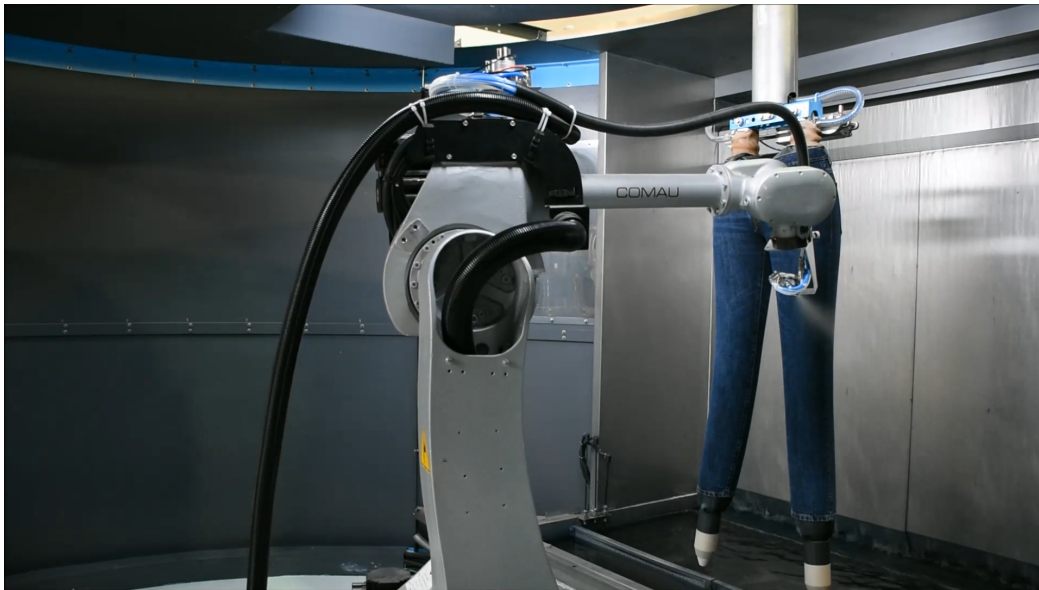
Figure 4.4: The robot in the Water Brush system executing a trajectory.
