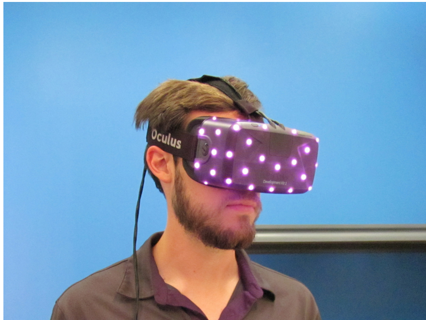
Figure 1.7: The array of infrared leds on the Oculus Rift DK2.
