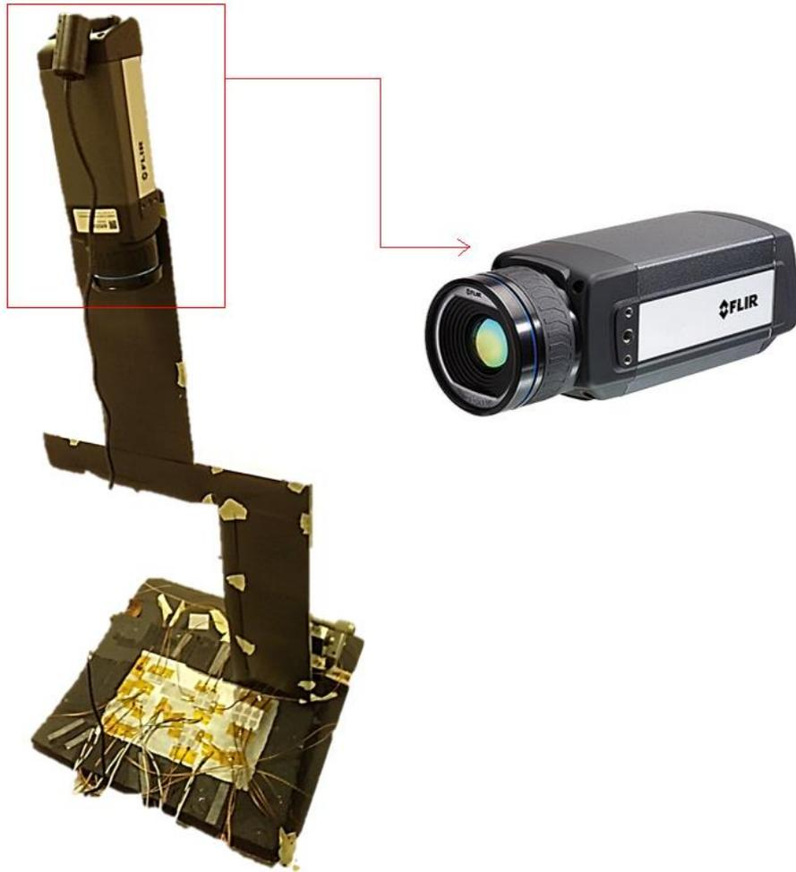
**Fig. 51** Infrared camera: installation for acquiring temperature data from the cold plate
