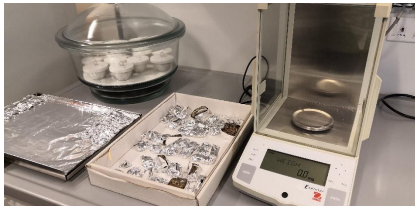
Figure 13: Foils containing samples ready to be weighted. Crucible samples cooling off in the background
