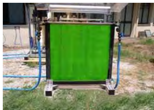
Figura 1.8. Fotobioreattore flat-panel ( http://deltafarmpress.com/mag/farming_commodities_future_algae/index.html ).
