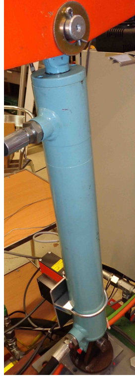
Figure 2.8: Hydraulic Cylinder MIRO C-10-60
