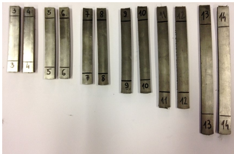
Fig. 25 Couples of samples with different thickness reduction
