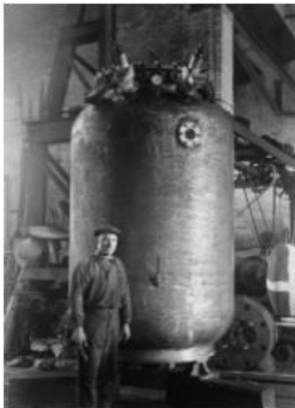
Fig. 2 Autoclave in 453S for gunpowder production [2]
