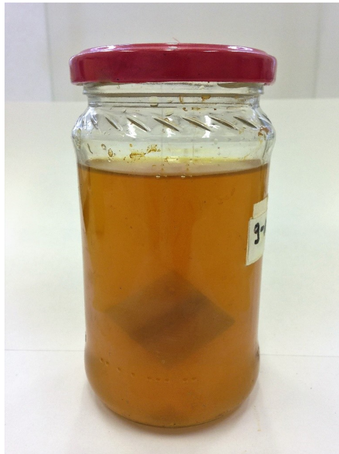
Fig. 30 Glass container test with the 40% deformed sample totally immersed in the Ferric Chloride Solution
