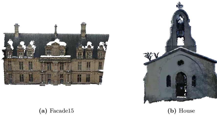
Figure 3.3: Point Clouds obtained with the structure from motion technique
