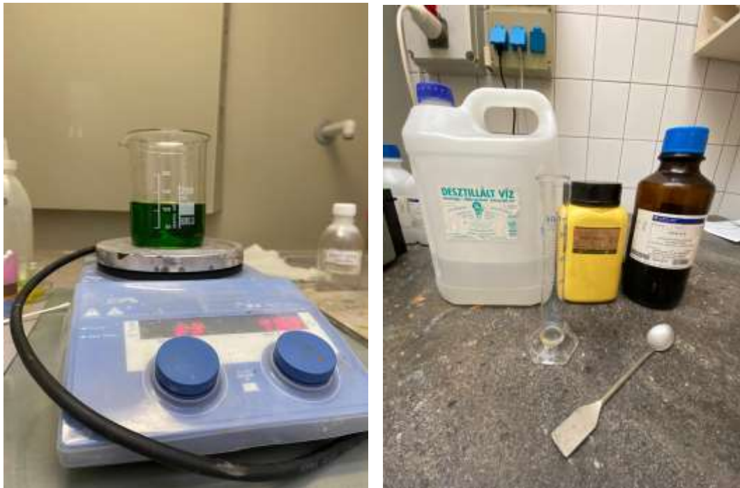
Figure 20 on the left: Magnetic agitator and the mixing step
