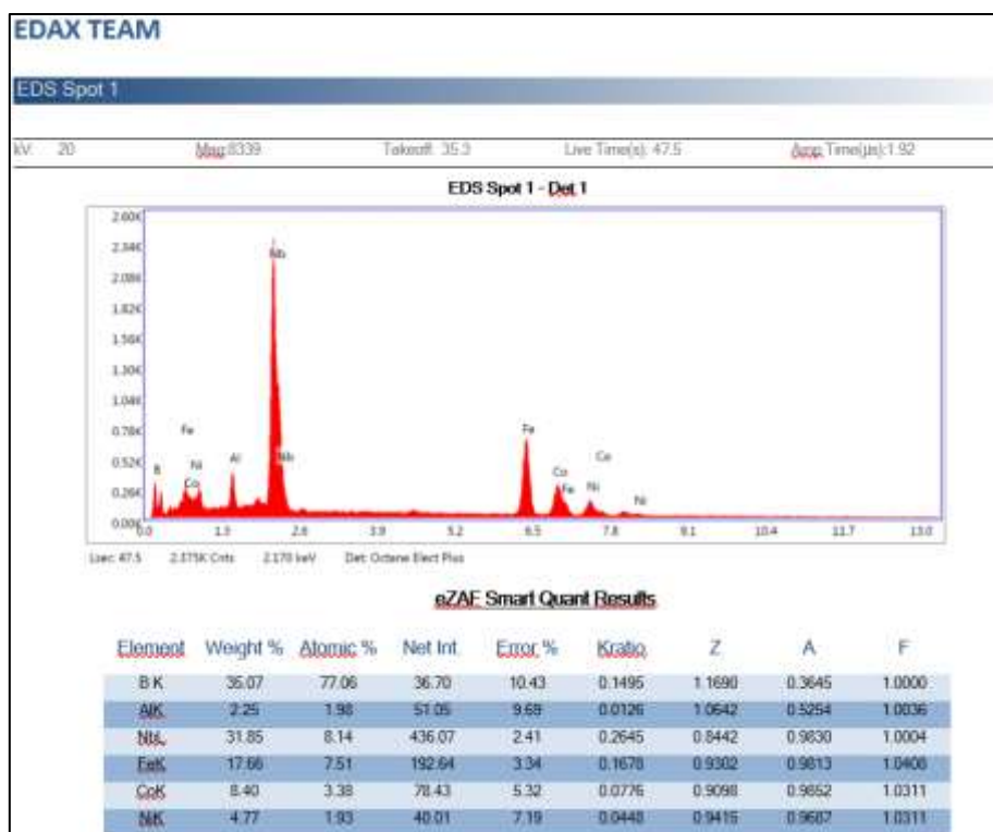
Figure 34 EDS spot composition analysis of the original sample
