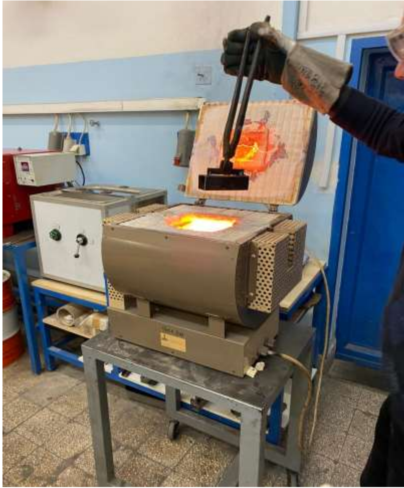
Figure 12: Homogenizing step of the heat treatment
