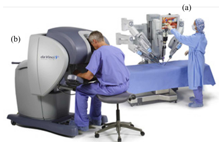
Figure 2.1: Da Vinci set up an operating room. (a) Follower robot, (b) leader robot.
