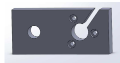
Figure 3.7: Solidworks CAD of adapter to attach the sensor to the articulated arm.
