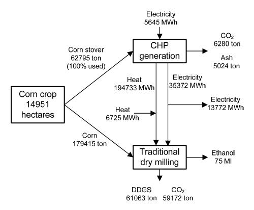
Figure 3.10: Overall process - Configuration 4
