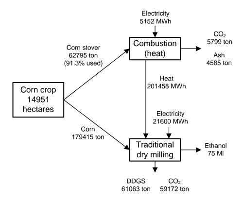
Figure 3.7: Overall process - Configuration 1
