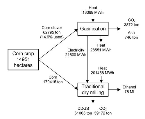
Figure 3.13: Overall process - Configuration 7
