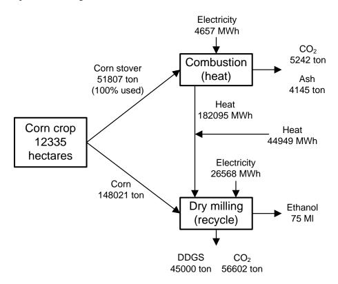
Figure 3.8: Overall process - Configuration 2
