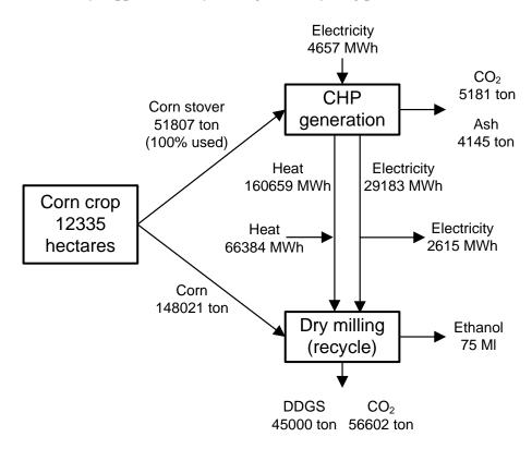
Figure 3.11: Overall process - Configuration 5
