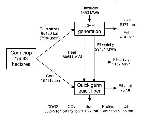
Figure 3.12: Overall process - Configuration 6
