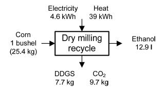
Figure 3.2: Model of dry milling whit recycle process
