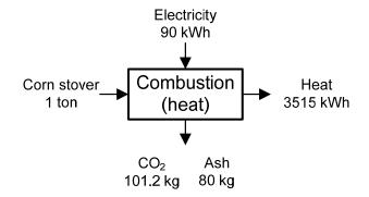
Figure 3.4: Model of combustion process for heat generation
