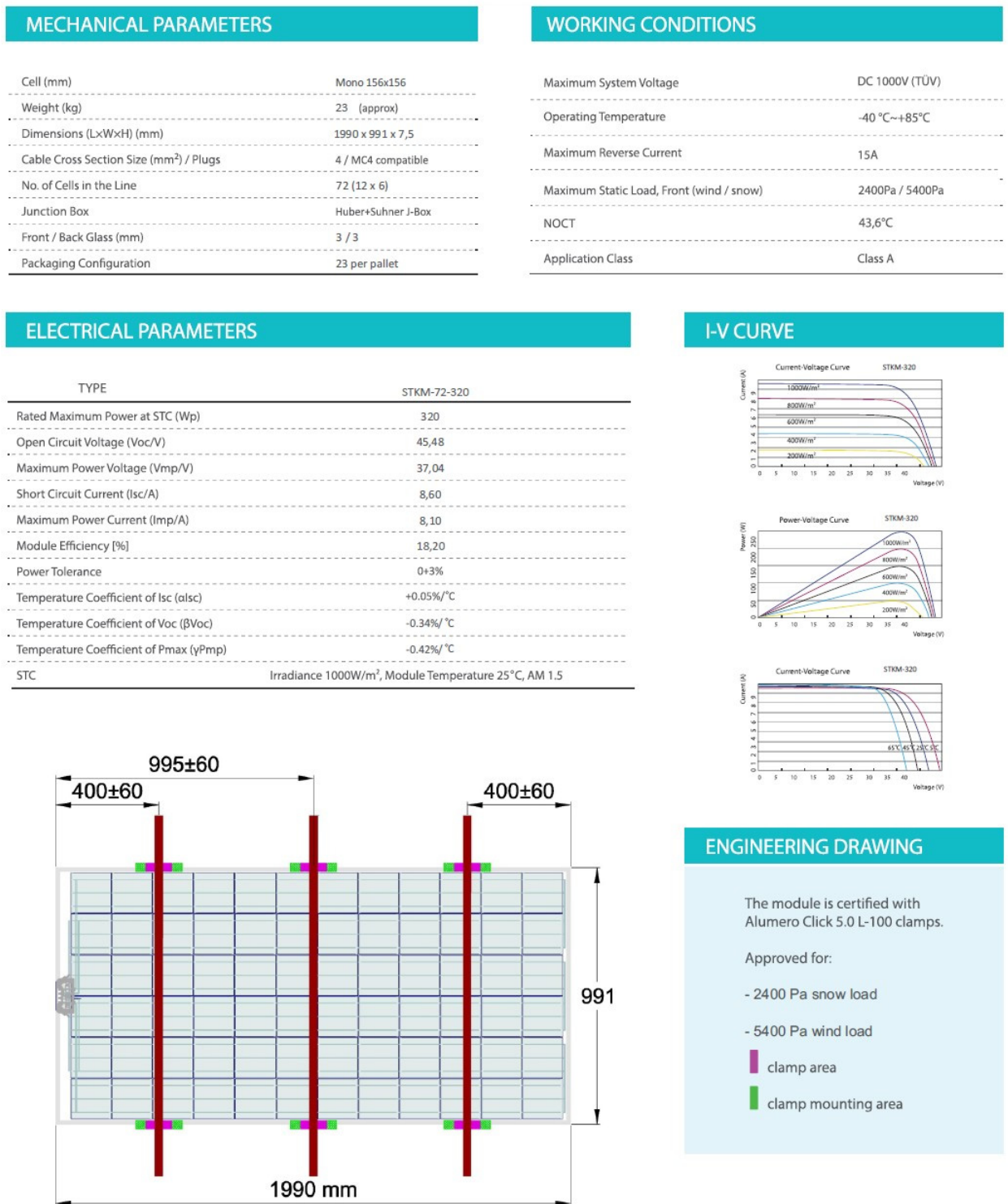
Fig. 2.6 - Datasheet of the selected PV module - "Solar Electric - STKM 320Wp Monocrystalline 72 cells module"
