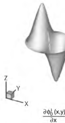
FIGURE 3.3: An MLPG shape function derivative along one direction.
