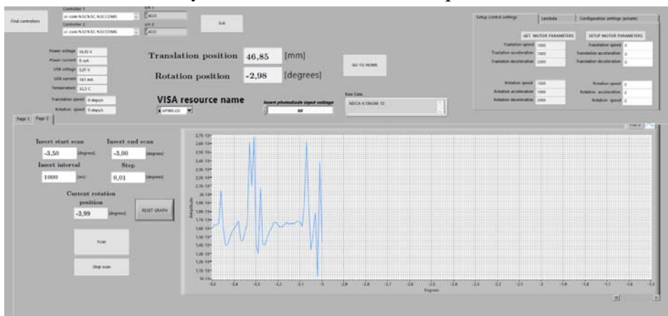
Figure 5.2: Measuring of current during a scan between two defined angles, with pre-selected time delay (in ms) and step value (in degrees) of the grating rotation.
