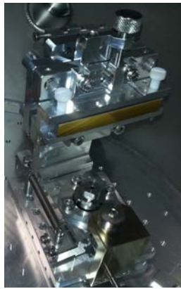
Figure 4.9: Toroidal gold coated mirror in the monochromator chamber.
