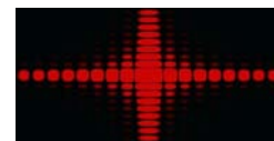
(b) Image obtained in a screen by a finite dimensions rectangular slit
