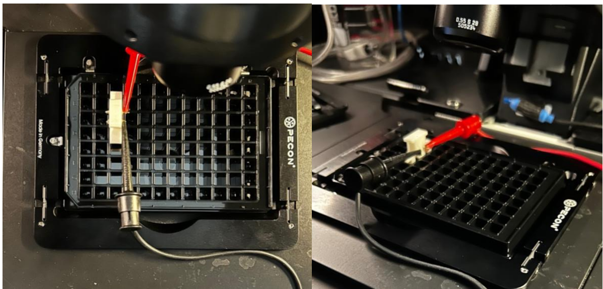
Figure 2.26: The \mu -Plate placed on the microscope stage. The electrodes are mounted into one of the wells and connected to the pulse generator.
