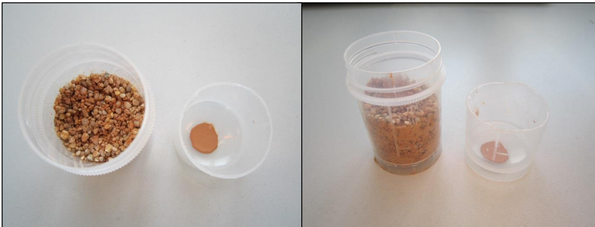
Figure 5-8 Percolation test: column and collector result after the fifth injection of 10 ml suspension at 100 g/L of red clay.
