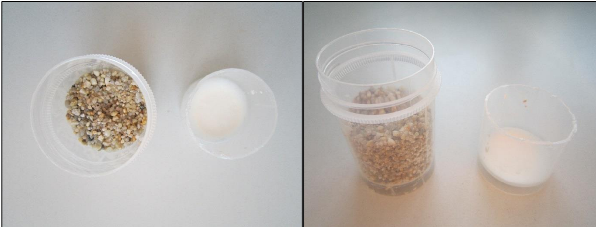
Figure 5-7 Percolation test: column and collector result after the fifth injection of 10 ml suspension at 80 g/L of kaolin.
