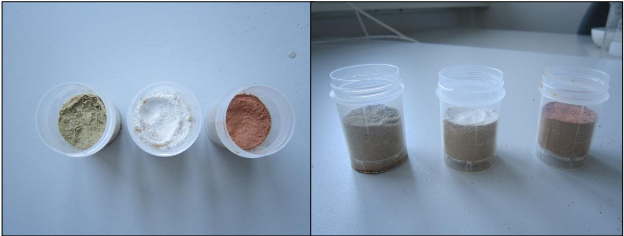
Figure 5-6 Examples of complete straining effect in fine sand media for bentonite (20 g/L), kaolin (30 g/L) and red clay (50 g/L) in column tests.
