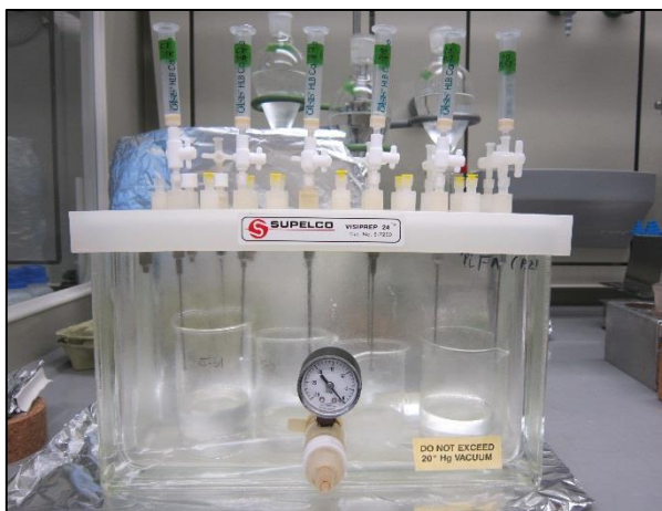
Figure 5-10 Solid Phase Extraction: conditioning step.
