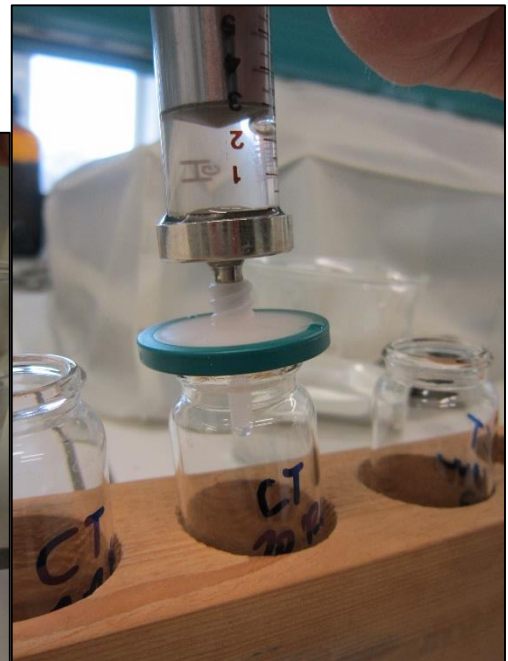
Figure 5-22 Filtration of the 10 ml extracted clay suspension aqueous phase.
