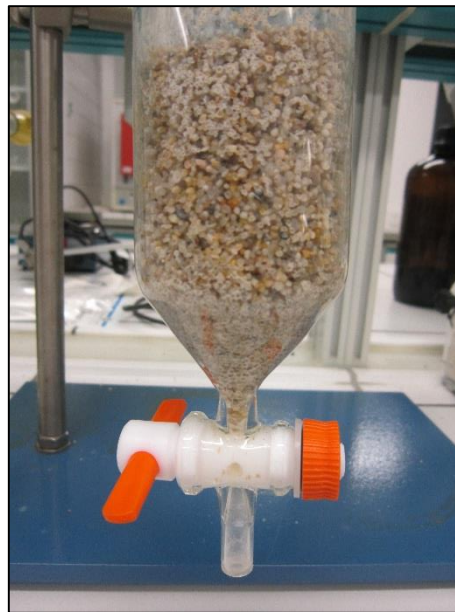
Figure 5-23 Example of straining effect on column. The bottom part of the column retained clay particles after the test end.
