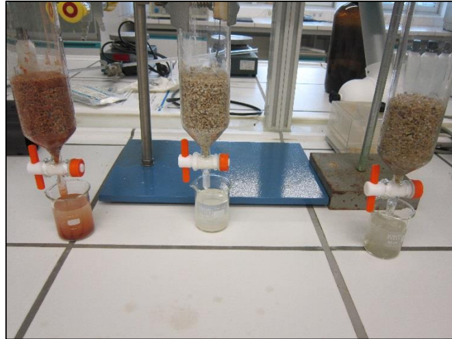
Figure 5-20. Column valves were opened after 24 hours of injection and clay suspension. Clays were then collected in flasks.
