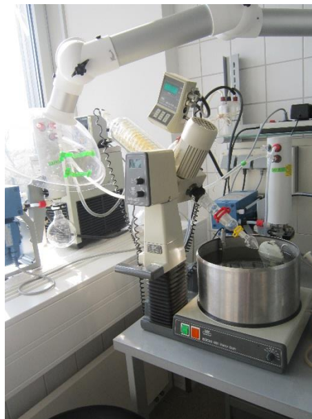
Figure 3-4 Rotavapor BÜCHI 461 Waterbath.
