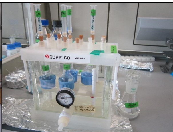
Figure 5-11 Solid Phase Extraction: elution step.
