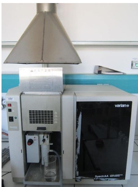
Figure 3-3 Varian SpectrAA 220 used for atomic absorption spectrometry for samples chemical analysis.
