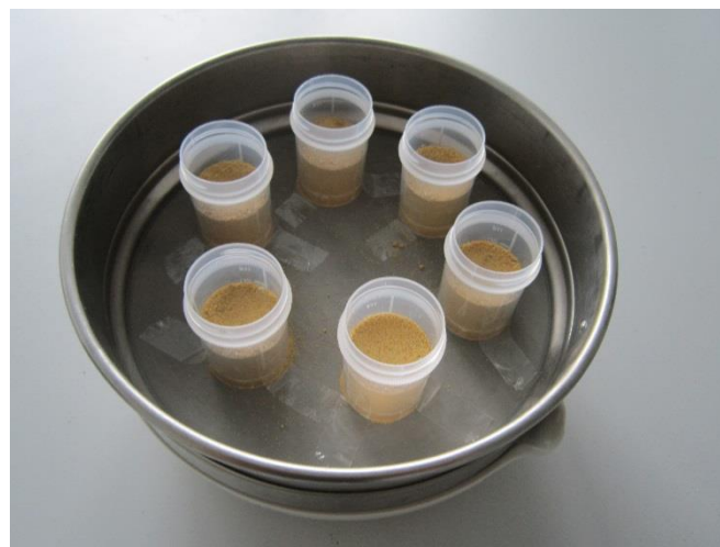
Figure 5-2 Example of test equipment: small columns fixed on 63 \mu\text{m} sieve and filled with sand.
