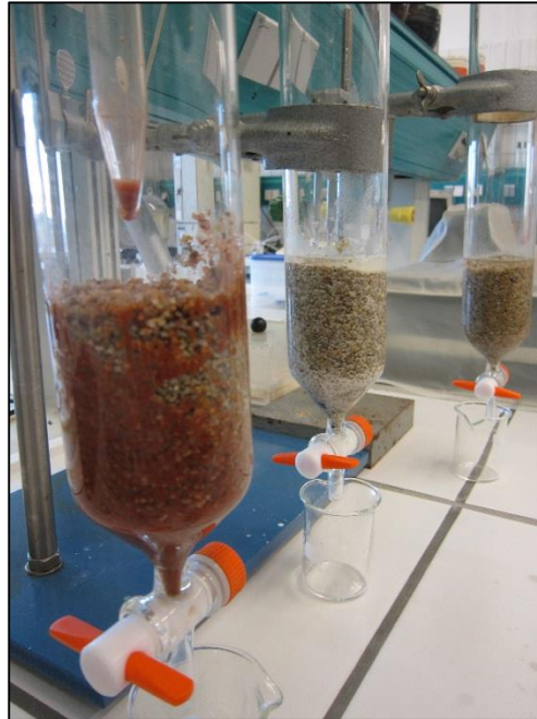
Figure 5-19 Injection of red clay suspension into the contaminated soil in column test.
