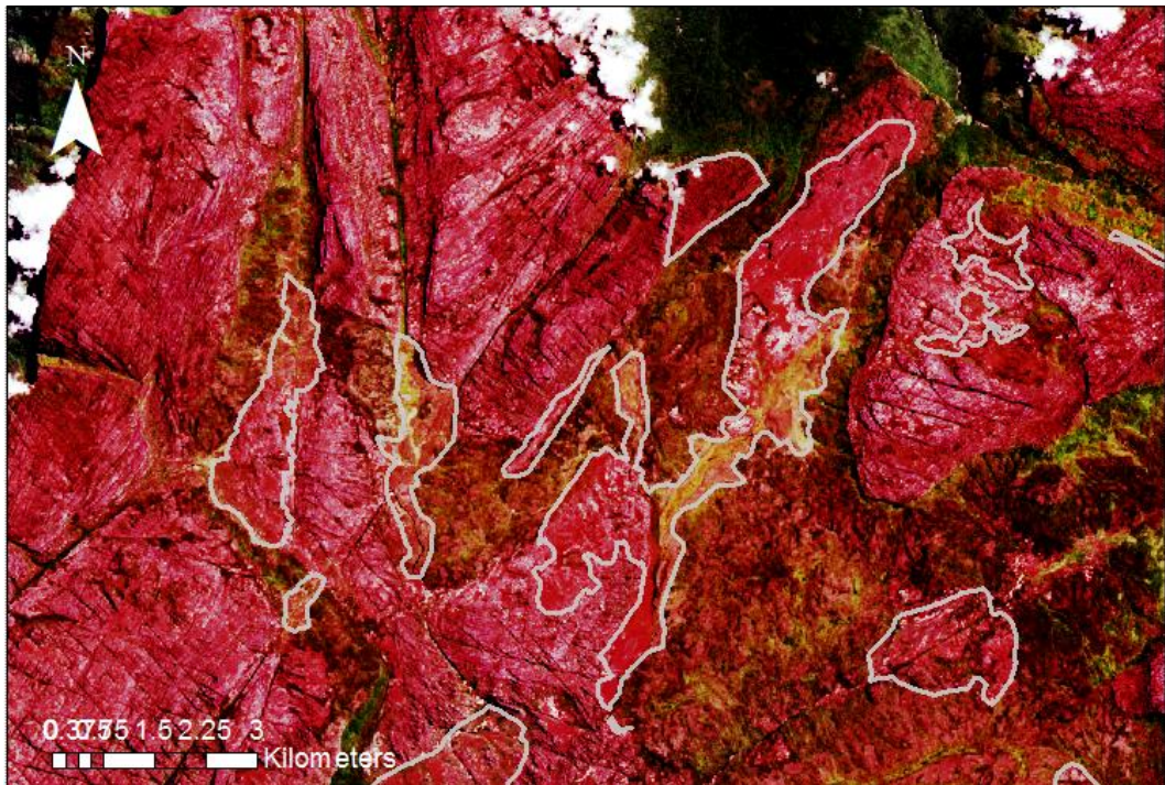
Figure 31. Detail of the central part of the Chimantà Massif, with, edged with the grey line, the portions interpreted as alteration.
