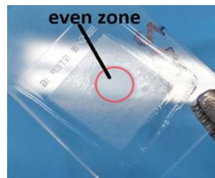
Fig.48: Pillars replica from droplet setup: we achieve an even replica only in the centre of the master, were bubbles could coalesce together more easily being in higher number, while peripheral areas are dotted in empty spaces.
