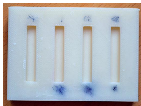
Fig.28: Die employed for swelling samples polymerisation.
