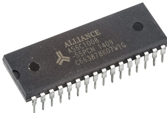
Figura 3.1.1: SRAM Alliance Memory da 1Mbit, 128000 byte x 8 bit, 32 Pin
