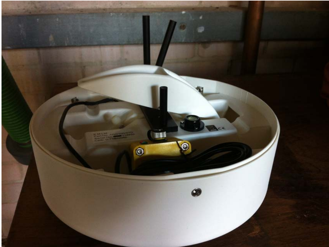
Figure 7: Tipping-bucket used for our research.
