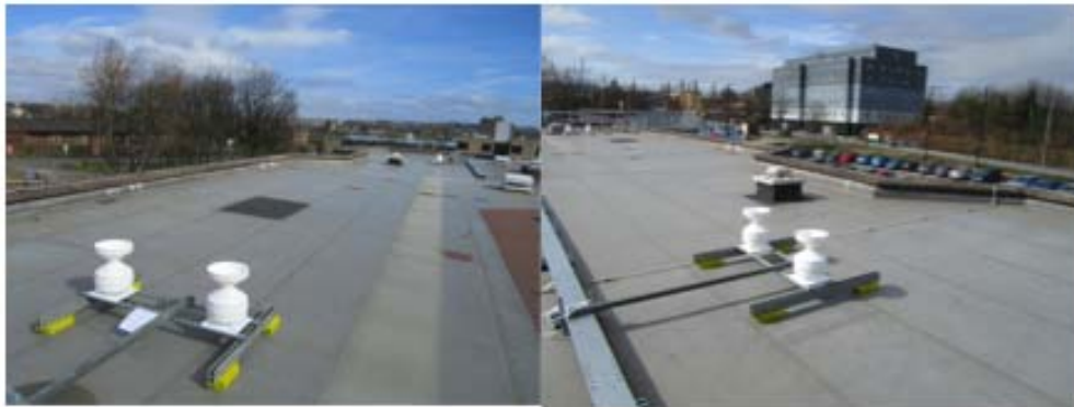
Figure 18: Rain gauges of point I and H, on roof of Student Central.
