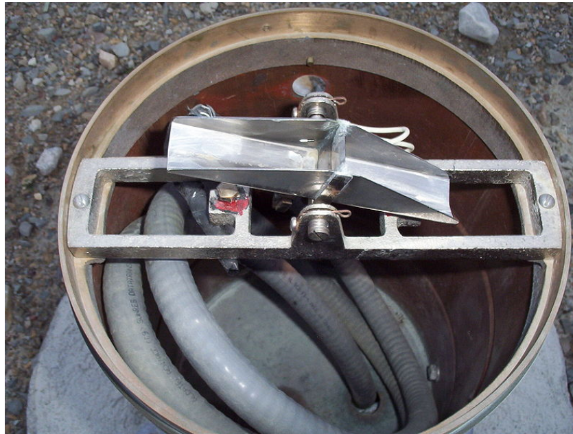
Figure 4: Tipping-bucket rain gauge, internal view.
