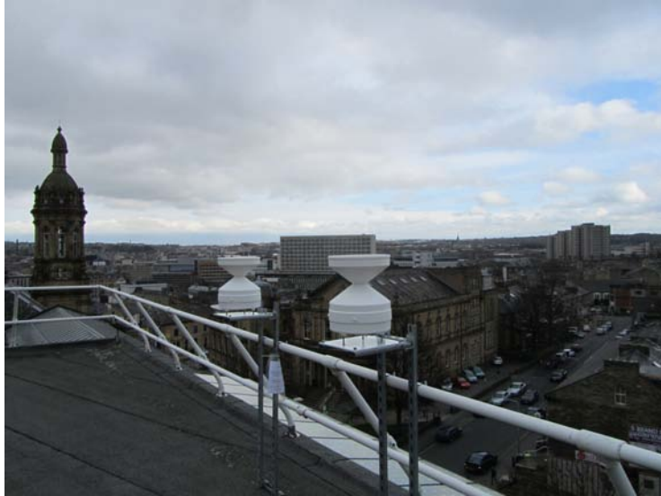
Figure 15: Rain gauges of point C, in Richmond building.
