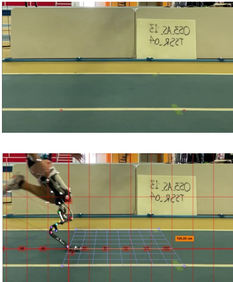
Figure 5.8. Red tape on the running lane (top); calibration grid, line and reference frame (bottom).
