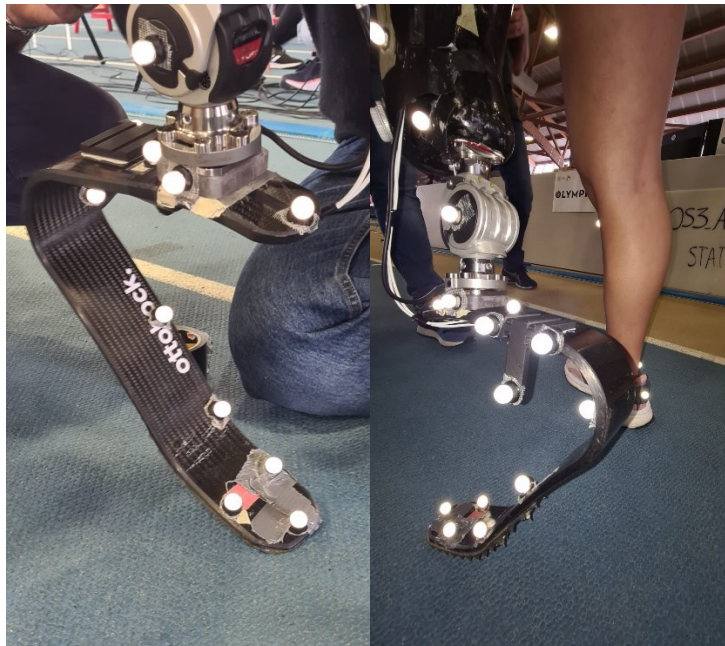
Figure 5.5. Detail of prosthesis' markers and pylon from the front (left) and rear (right).
