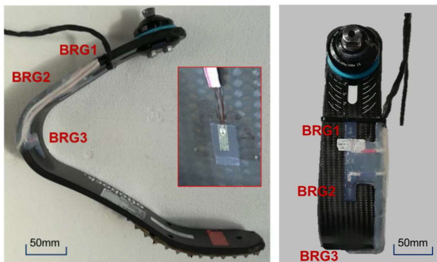
Figure 2.2. Instrumented Ottobock Runner CAT 4, developed by Petrone et al.
