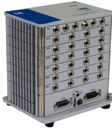
Figure 4.6. SOMAT acquisition unit.
