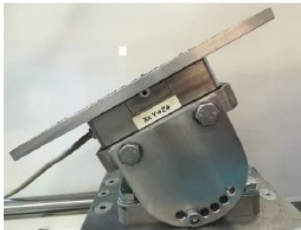
Figure 4.4. Horizontal sledge connected to the holed flange to replicate the angles of \theta_{SH} .
