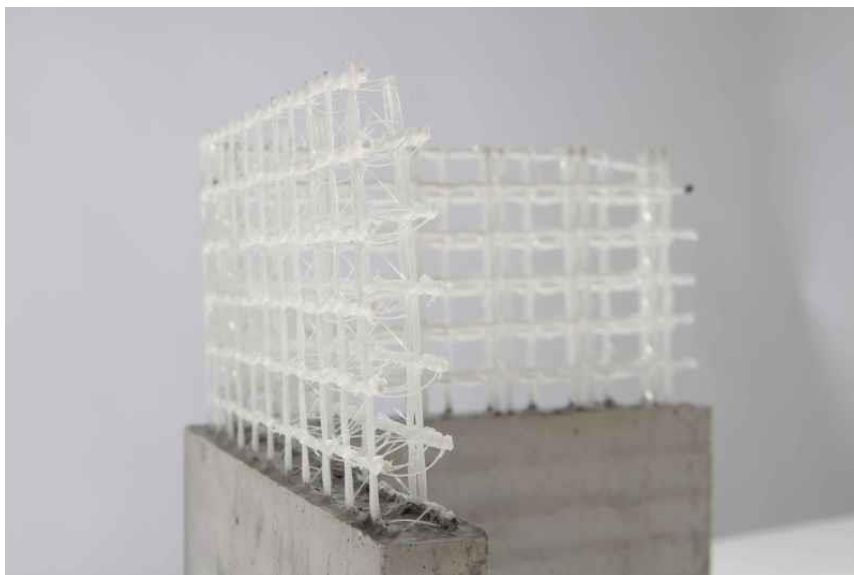
Figure 10 Two examples of textile fiber use for concrete flooring and wall
