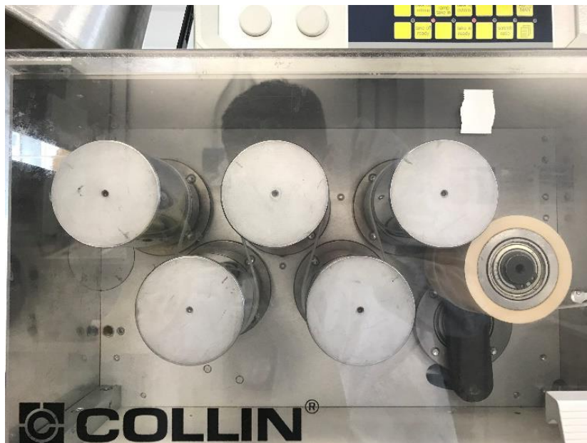
Figure 15 From above: extruder die (final part of the extrusion process), rolling process of the filament after the extrusion, particular of the rolls
