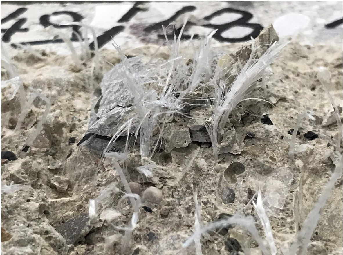
Figure 36 particular of fibers: some are completely frayed/ exhausted, others are still intact due to different behaviour during flexural test
