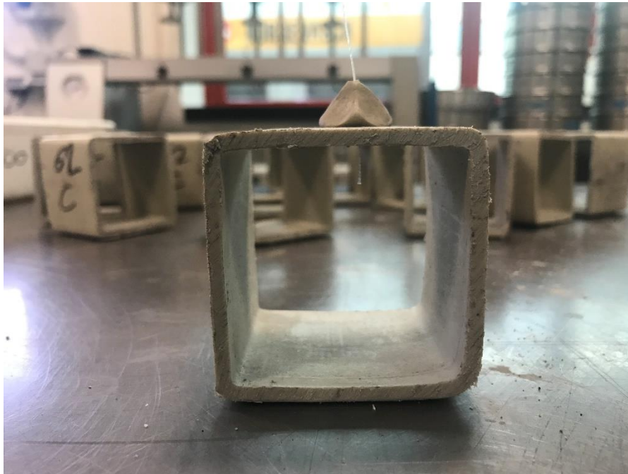
Figure 30 Exemple of a sample with the fiber attached on the top ready to be filled with mortar
