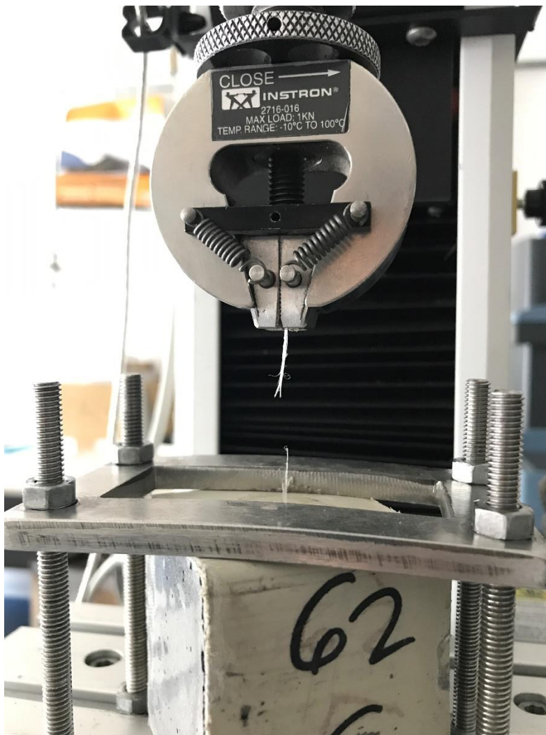
Figure 32 Setting of pullout test on Instron machine
