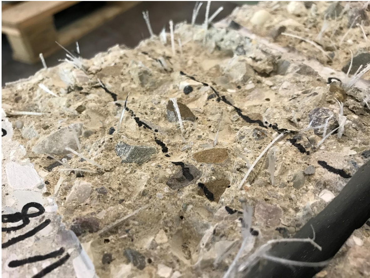
Figure 34 View of fibers on surface of cracked samples
