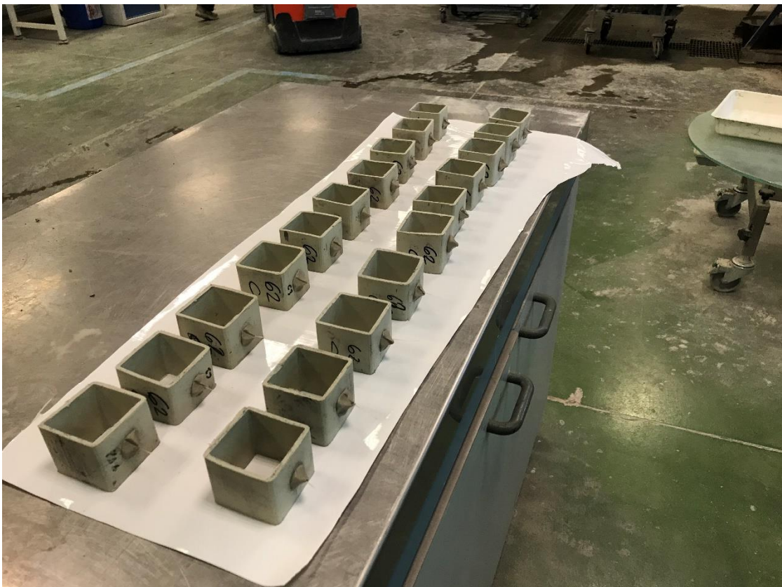
Figure 31 Steps of preparation for pullout test samples
