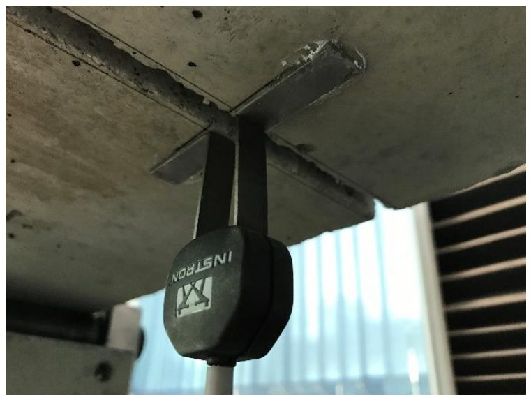
Figure 24 Setting of Instron machinery with three points flexion. Particular of the sensor under the sample
