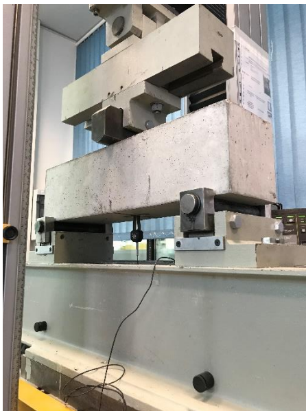
Figure 24 Setting of Instron machinery with three points flexion. Particular of the sensor under the sample
