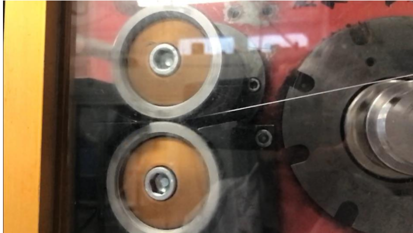
Figure 17 Particular of the filament passing through two rolls that give the geometry to the surface
