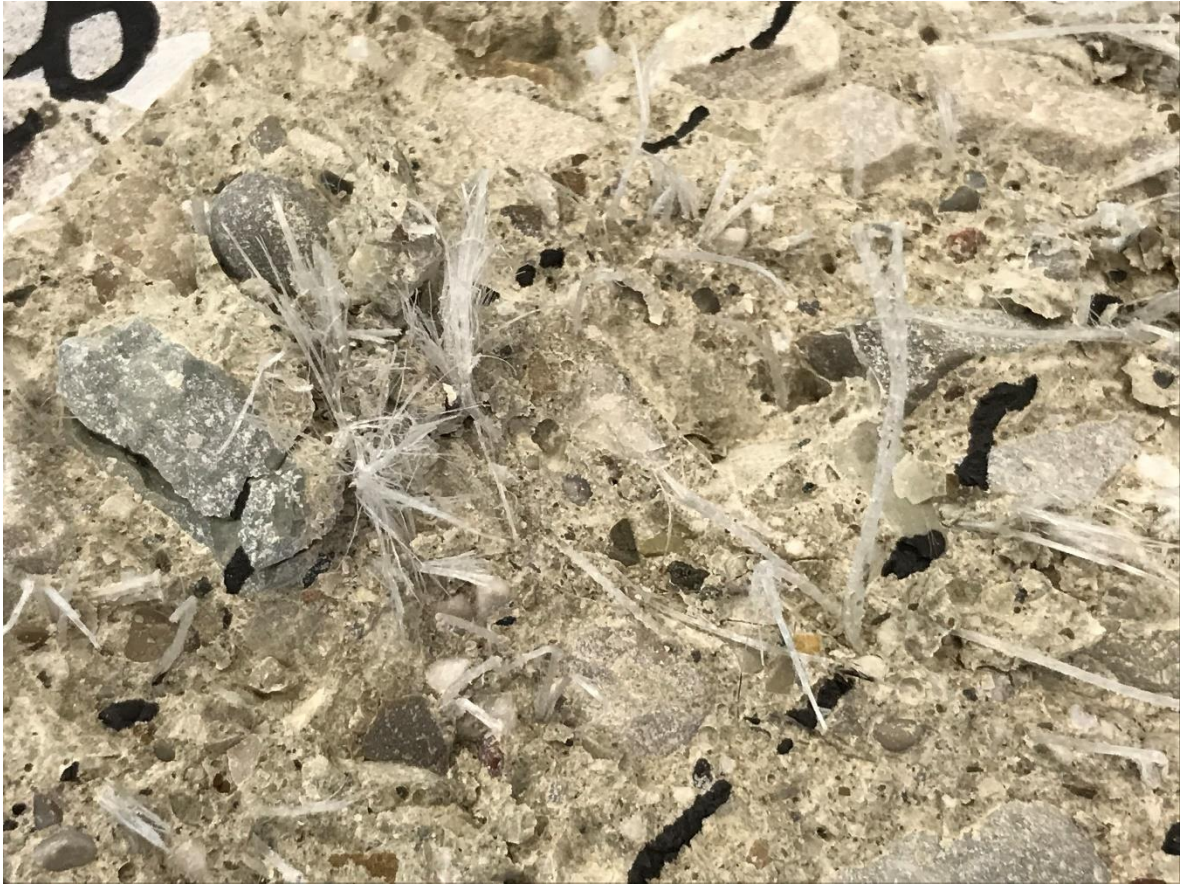
Figure 36 particular of fibers: some are completely frayed/ exhausted, others are still intact due to different behaviour during flexural test
