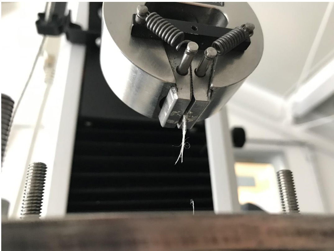
Figure 33 Closer look to setting of the clamp in pullout test
