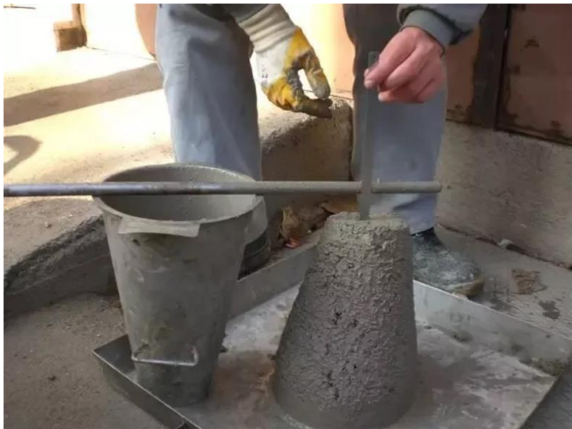
Figure 7 usage of Abram's cone
