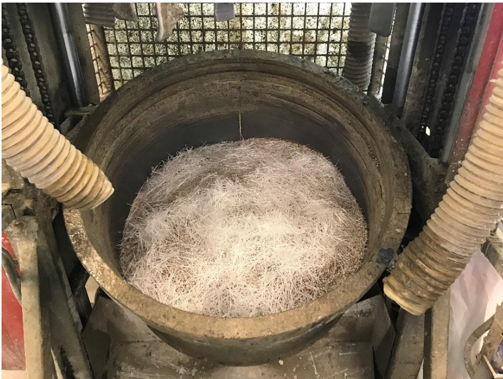
Figure 21 First stage of preparation FRC concrete before mixing
