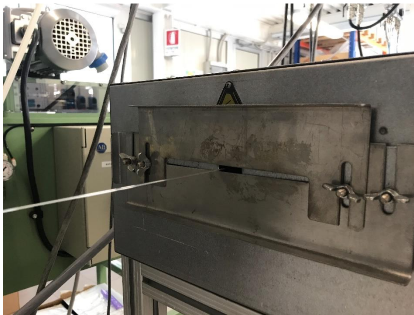
Figure 16 Particular of the filament coming out from the oven where hot temperature and continuous stretching force applied give the right diameter
