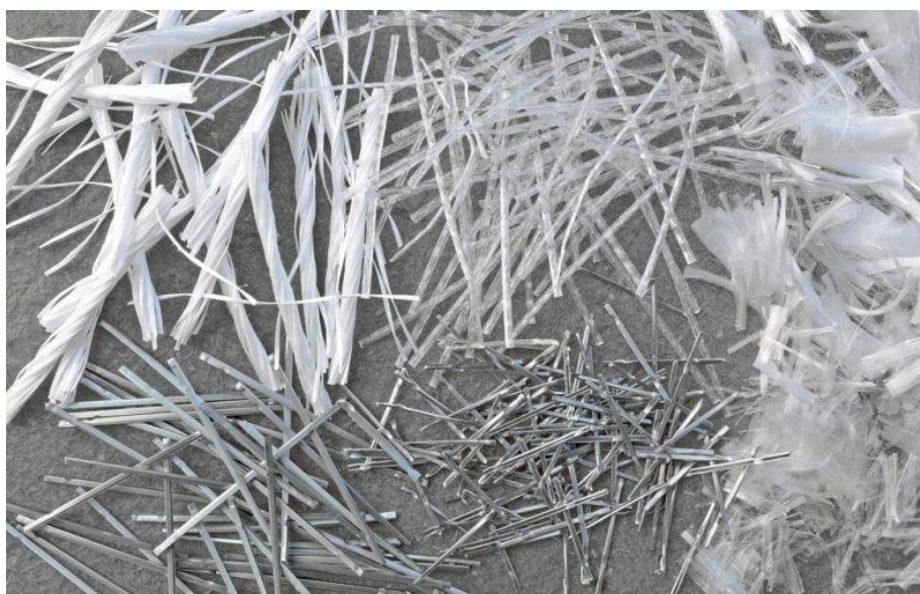
Figure 9 Different types of fibres used in FRC concrete
