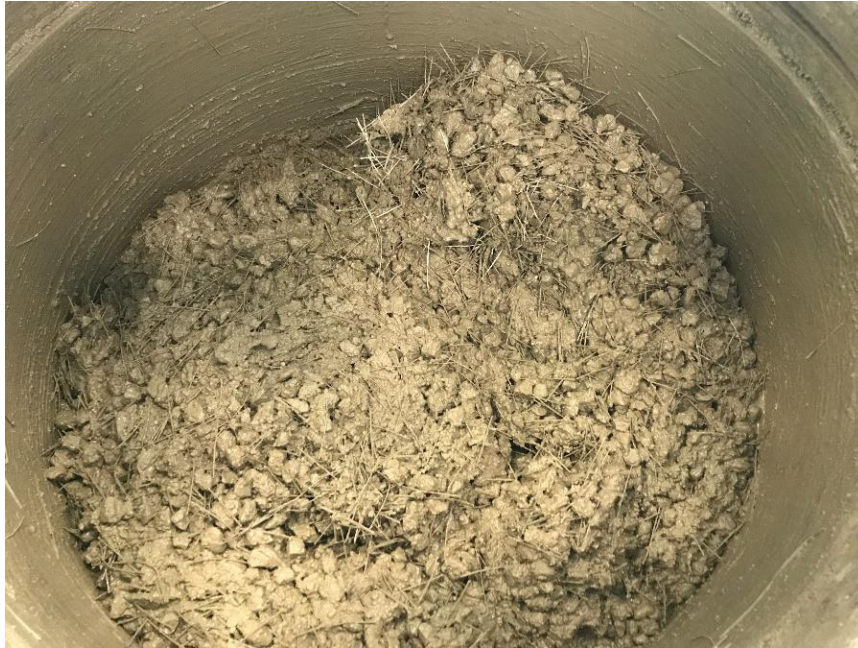
Figure 22 First stage of preparation FRC concrete after mixing
