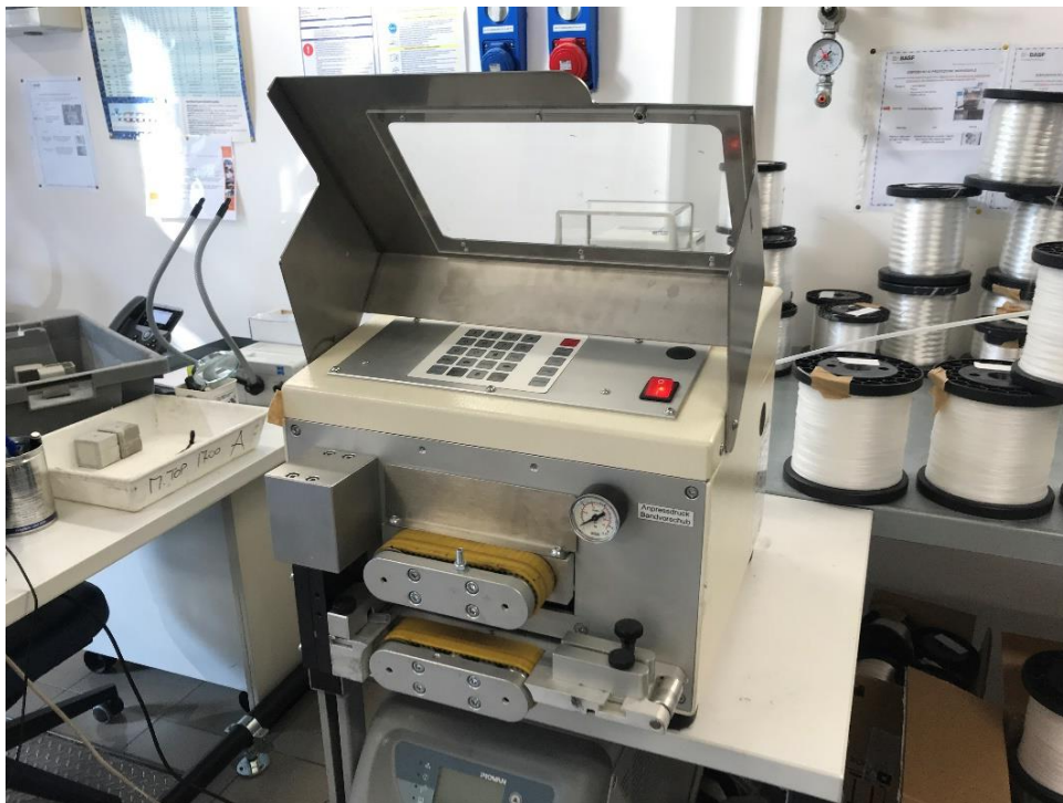
Figure 18 Machinery used for cutting filament operation
