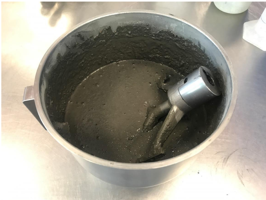
Figure 29 Mortar mix after mixing
