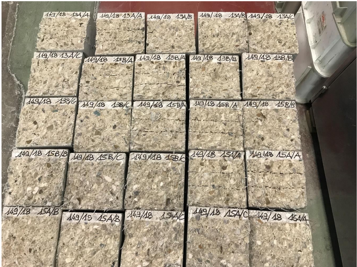
Figure 35 Set of tested samples after final cracking
