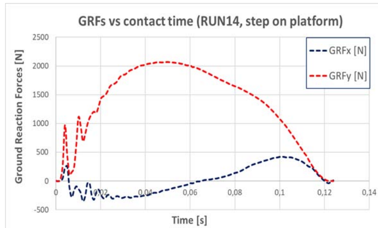
Figure 4.11: Ground reaction forces in the Ground reference frame (step on platform, RUN14)
