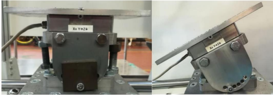
Figure 2.6: Horizontal system of inclination [17]
