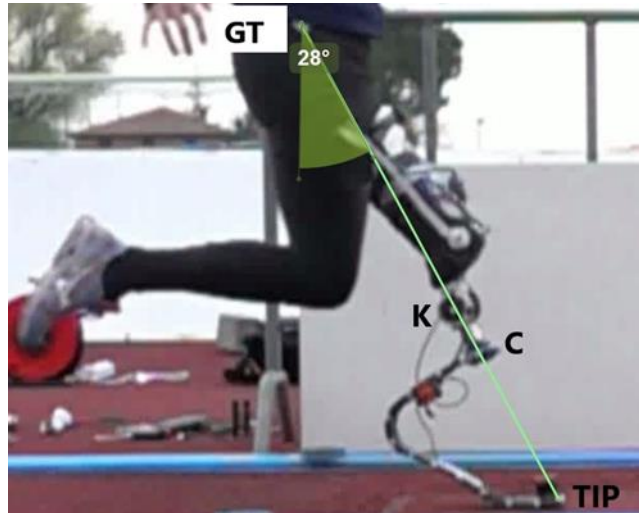
Figure 5.1: Heel Strike instant (RUN14). Note the 28^\circ angle between the perpendicular to the ground and the segment passing through the greater trochanter (GT) and the tip of the prosthesis (TIP)
