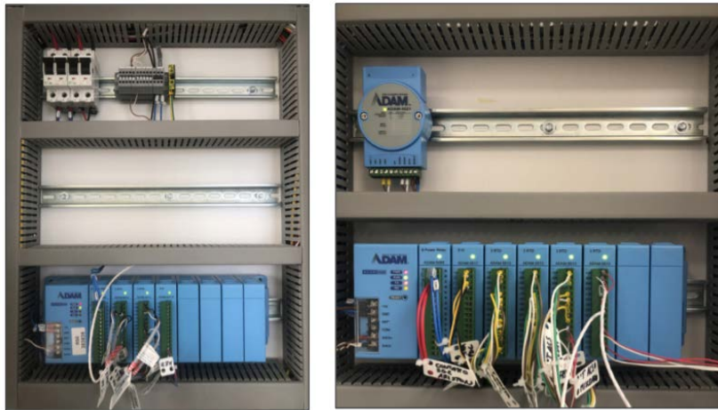
Figure 2.5: Data acquisition modules Advantech ADAM 5000 and 4000.
