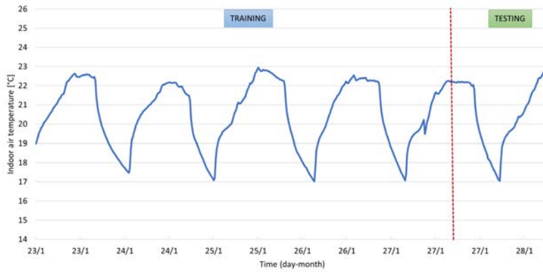
Figure 5.7: Mean indoor temperature in Winter 3 in training (4 days) and testing period (1 day).
