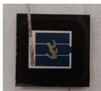
*Figure 3.3: Initial delamination induced by EVA.*
