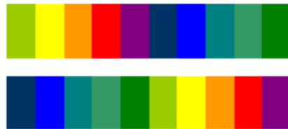
Figure 2-3 Complementary colours: the upper row represents the solution colour, the bottom one represents the fraction of light absorbed by the solution [25].
