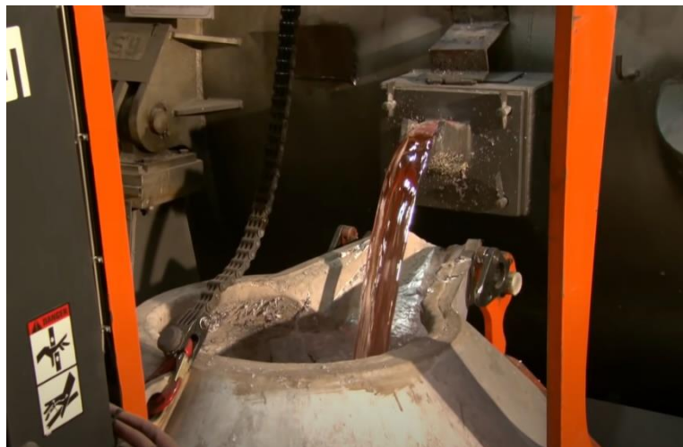
Figure 15: Pouring operation at a casting plant. Note the height at which the metal is being poured from the furnace into the transfer ladle.
