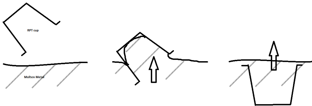
Figure 31: Immersion of the RPT cup "head first" in order to gently push the oxides to the walls of the cup and avoid turbulence
