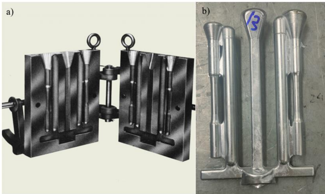
Figure 32: a) example of Sthal Mold design for tensile test bars casting, in all similar to the one used in the experiment. b) example of casting obtained from the Sthal Model once the melt solidified.
