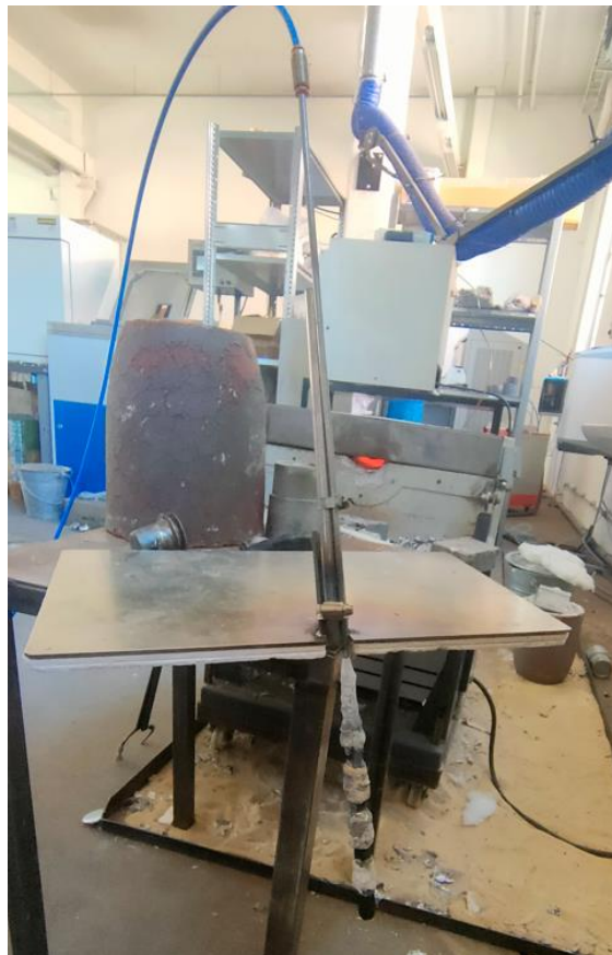
Figure 29: Graphite lance mounted on refractory cover and connected to gas inlet
