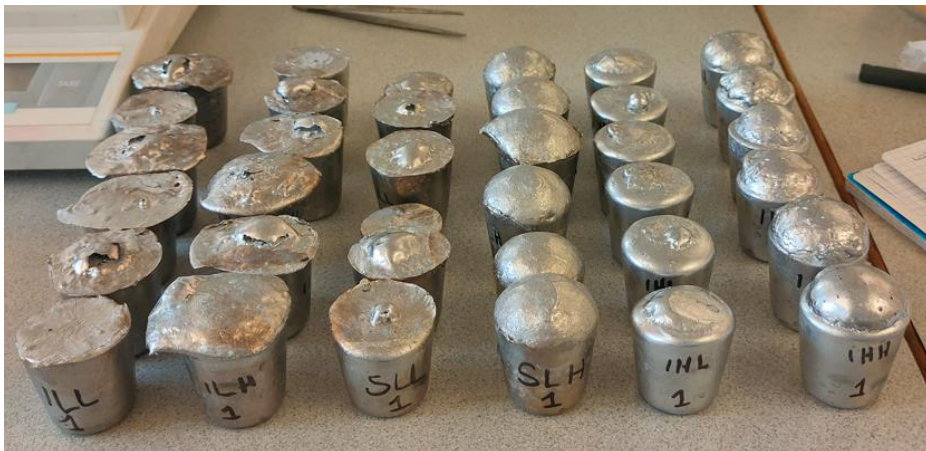
Appendix 7A: Overview of all the RPT samples before the cutting operation. From left to right: ILL, ILH, SLL, SLH, IHL, IHH
