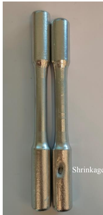
Figure 35: Example of two tensile test bars, one without shrinkage and one with shrinkage
