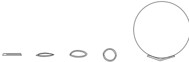
Figure 52: Overinflation of a bifilm by hydrogen gas [19]
